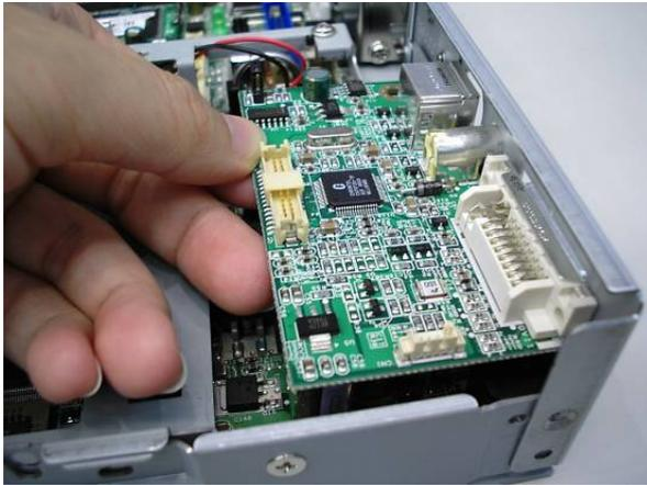
a. Insert the DVO board into the I/O bracket.
