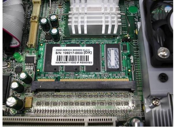
b. Push the card down gently until two metal latches on the side of the slot click into place.
