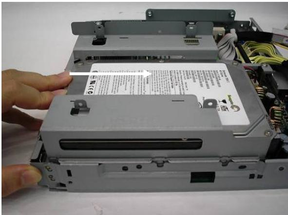
g. Slide the 3.5" HDD to remove it.
