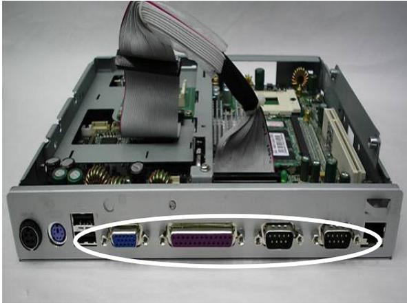
c. Remove the hex secures (8) to remove the I/O bracket.
