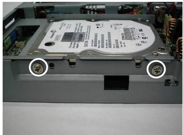
b. Remove the screws (2) that secure on the slim HDD.
