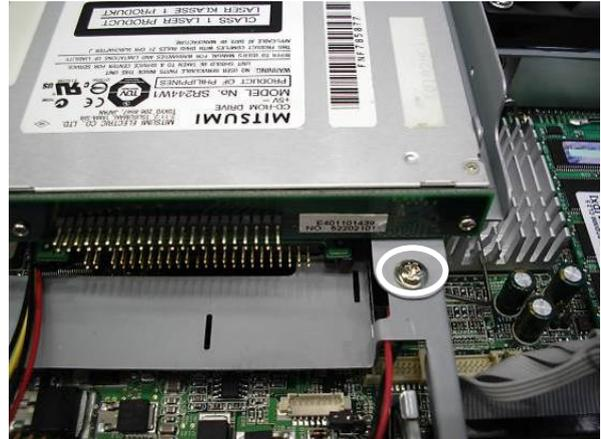
f. Remove the screw (1) to remove the bracket.
