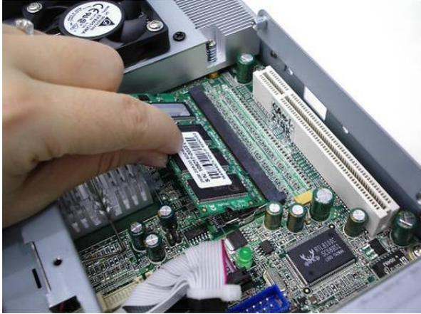
a. Install DDR Memory by inserting it into the slot.
