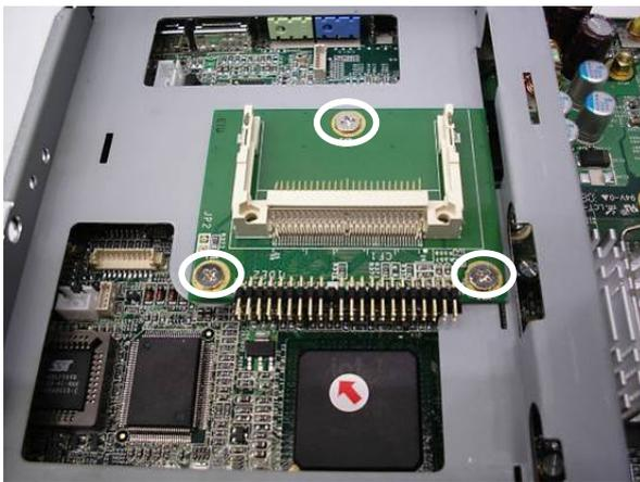
c. Remove the screws (3) that secure on the board.
