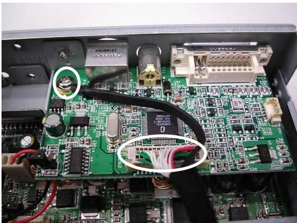
c. Tighten the screw with the ground cable. Then, connect the DVO cable (1).
