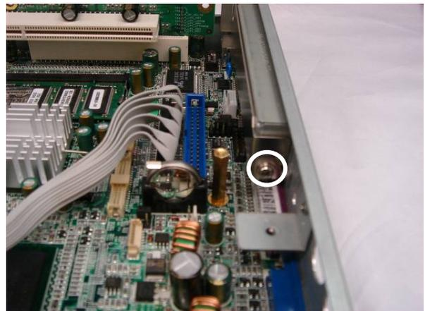
d. Remove the screw (1) that secures the PCI bracket.
