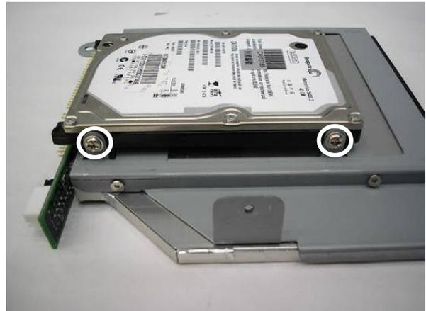
h. Remove the screws (2) to remove the slim HDD.
