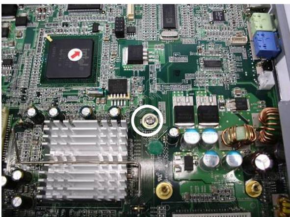
g. Remove the screw (1) that secures on the motherboard.
