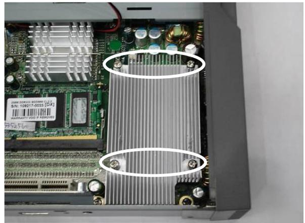
d. Remove the screws (4) that secure on the heatsink.
