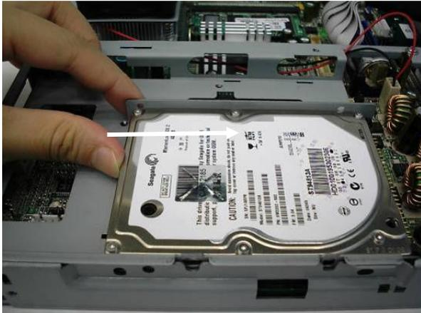
c. Slide the slim HDD to remove it.
