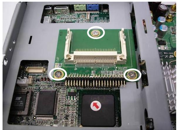
f. Remove the screws (3) that secure on the board.
