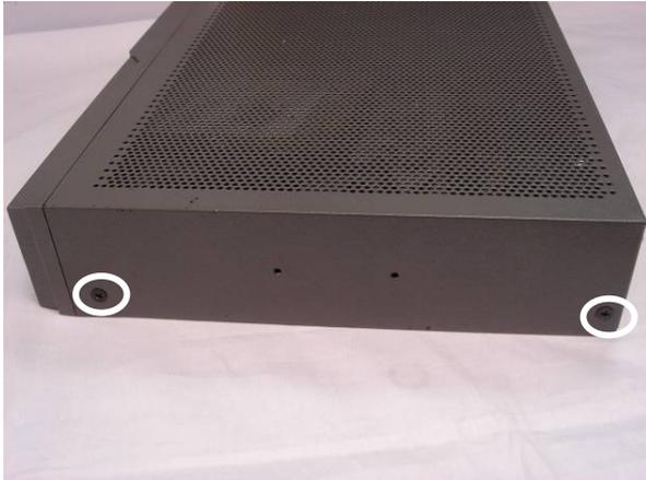
a. Remove the screws (4) (two on each side).
