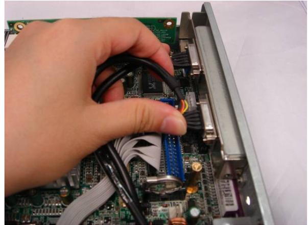
f. Insert the COM port cables into the slot.
