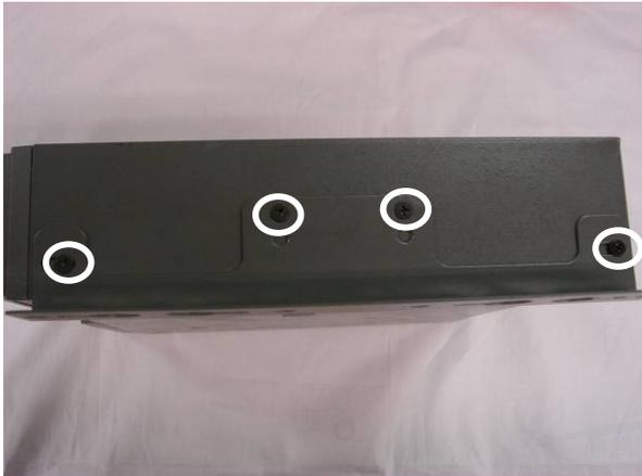
c. Tighten the screws (8) (four on each side).
