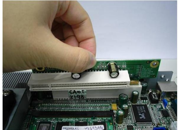
d. Remove the PCI slot.
