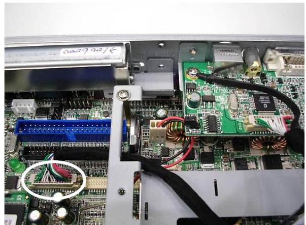
d. Connect the cable (1) on the motherboard.
