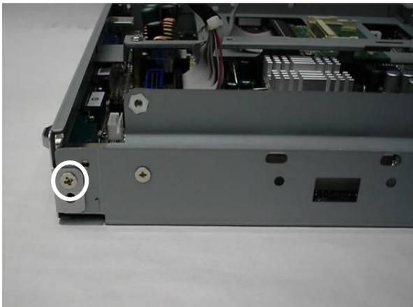
a. Remove the screw (1) that secures on the I/O bracket.
