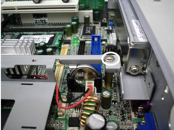
a. Remove the screw (1) that secures on the bracket.
