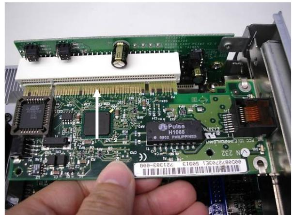
b. Insert the PCI card into the slot.
