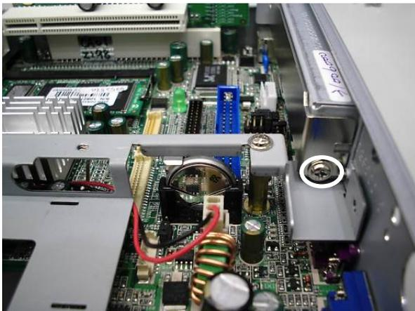
a. Remove the screw (1) that secures on the bracket. Then, remove the bracket.
