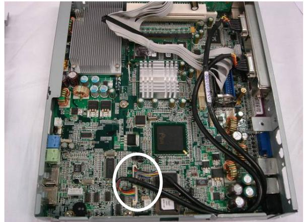
h. Connect the cables (2) (Refer to 6. Connectors & Jumper Settings).
