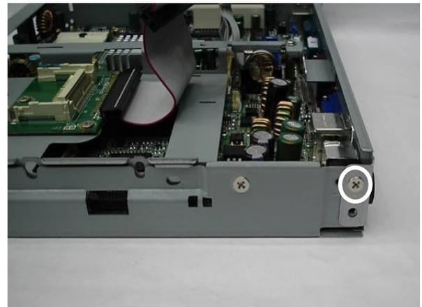
b. Remove the screw (1) that secures on the I/O bracket.
