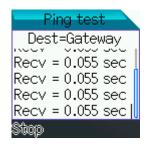
the test location. On the contrary, when the number of times WiFi phone sends signals is a lot more than the test location sending back signals, it indicates there is connection exception between WiFi phone and the test location.
