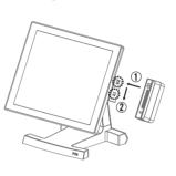
Please close I/O cover after inserting the cable into COM6/USB port of I/O ports.
