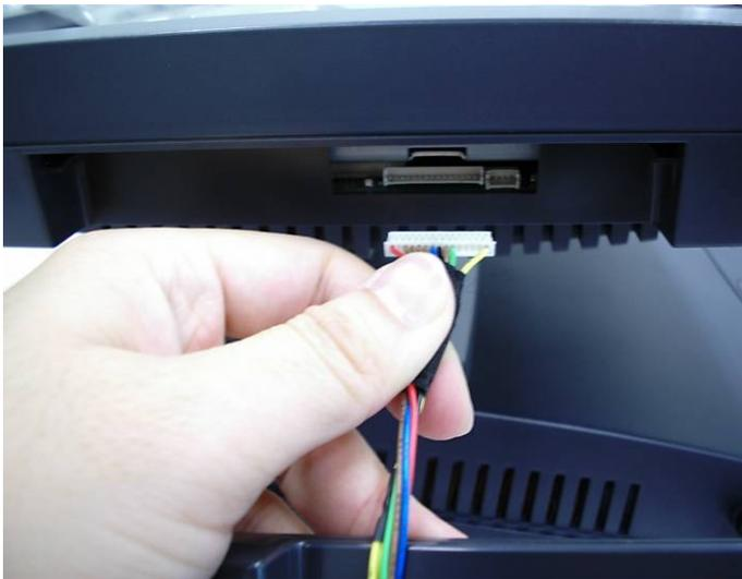
c. Connect the MSR connector on the right side of the system.
