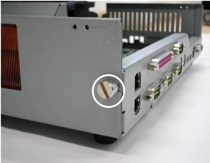
e. Remove the screw (1) on the left side.
