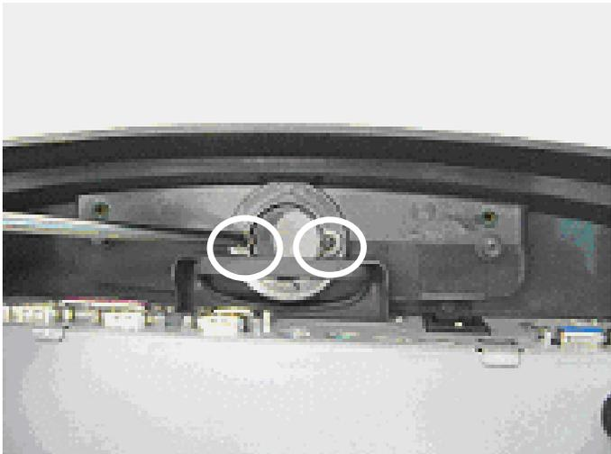
f. Tighten the screws (2) to fix the stand base.
