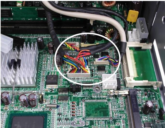
c. Disconnect the cables (4) as shown in the picture.
