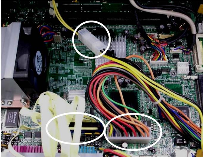
b. Disconnect the cables (3) as shown in the picture.
