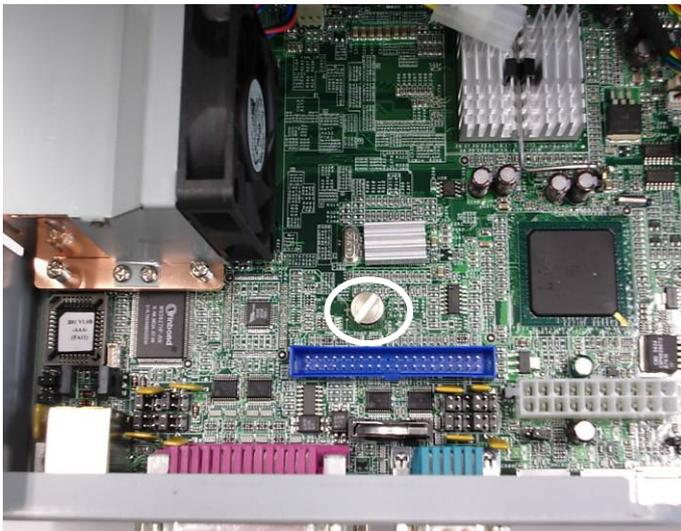
f. Remove the screw (1) on the motherboard.
