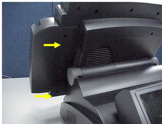
Push into the MCR module at the right side of System LCD Module then lock it with two screws.
