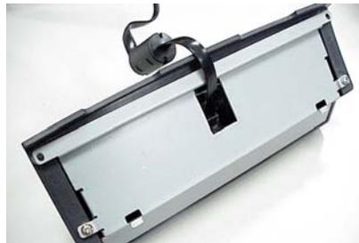
b. Insert the other end of the RS232 cable into the RJ45 connector of the Customer Display module.
