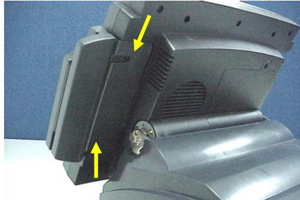
a. Push into the MCR module at the right side of System LCD Module then lock it with two screws.
