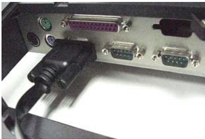
a. Insert the RS232 cable into any of the Com ports.
